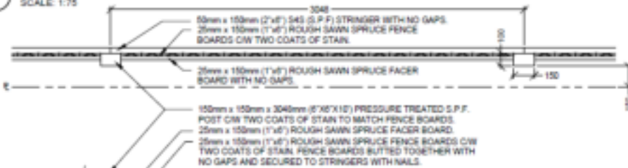
1800mm HT. STANDARD WOOD SCREEN FENCE STEP DOWN SCALE: 1:75
