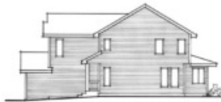
Inappropriate corner treatment
